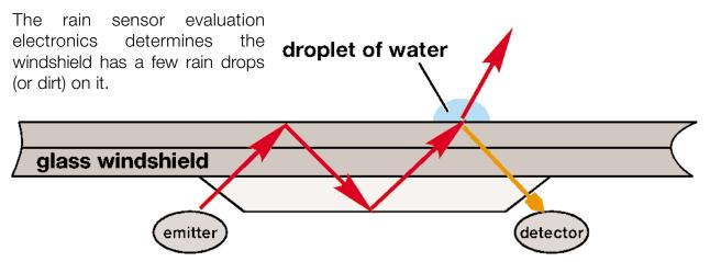
The intensity of the returned infra red beam diminishes proportionally with an increase of water droplets. The rain sensor control module generates a signal proportionate to the amount of rain on the windshield and broadcasts it to the GM III via the K bus.
